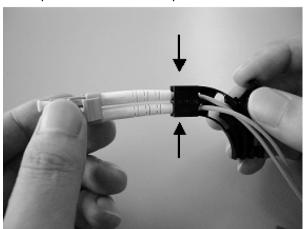
3 Hold the connector and protective holder, and press in the connector direction.
