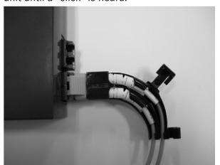
⑥ Insert the other connector into the IN side (top) of the unit until a "click" is heard, and catch the two cords together into the cord holder.
