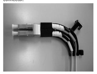
(5) Remove the dust cap, and insert the connector, onto which the protective holder has already been mounted, into the OUT side (bottom) of the unit until a "click" is heard.
