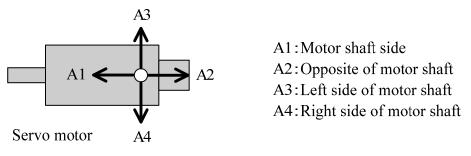
(Note) Depending on the situation such as installation environment or combination of cables and connectors, there is a chance not to complete installation. (Even though it's mentioned above) Please make sure the cable lead out direction before your purchase.
