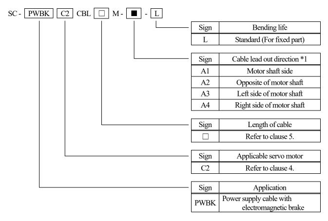
\*1:Cable lead out direction (View from cable insertion direction)
