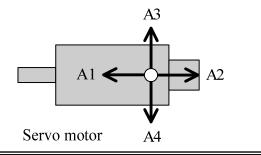
A1: Motor shaft side A2: Opposite of motor shaft A3: Left side of motor shaft A4: Right side of motor shaft
