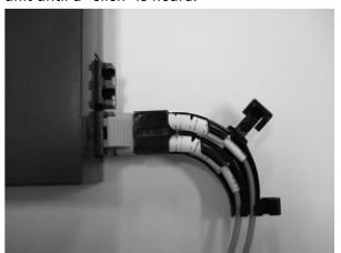
⑤ Insert the other connector into the IN side (top) of the unit until a "click" is heard, and catch the two cords together into the cord holder.
