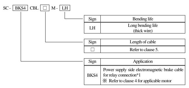
\*1 Please use it with power supply side electromagnetic brake cable. Refer to clause 6 for confirming the combination and cable length.
